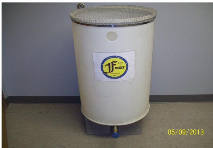
A rain barrel is a water tank used to collect and store rain water runoff, typically from rooftops via rain gutters. A collection system can yield 623 gallons of water from 1 inch of rain on a 1,000 sq. ft. roof. Stored water can be used for watering gardens, etc. and help with the conservation of water. If you would like to win this rain barrel, complete the form below, detach it and return it to City Hall. Good Luck!
